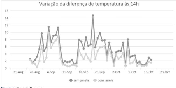
Graph of temperature difference at 2 PM in the two prototypes between August 27th and October 18th, 2021
