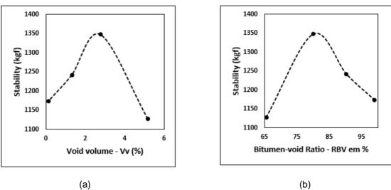
Figure 5 - (a) Stability versus %Vv / (b) Stability versus %BVR
