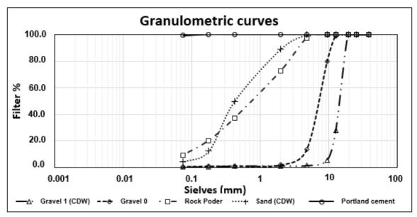
Figure 1 - Particle size analysis of the aggregates used in the present study
